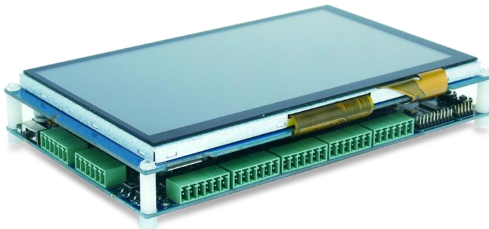
MYD-J335X-V2 Board with MY-TFT070TPCV2 7-inch LCD Module
