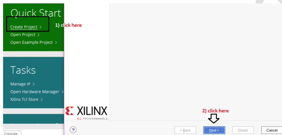
Figure 2. 1 : Starting a Project in Vivado
