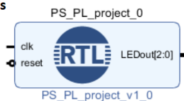
Figure 3. 8: VHDL entity in block form
