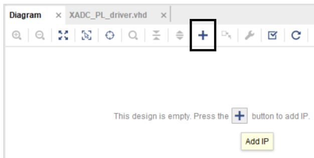
Figure 10. 4: Adding an IP to the Block Design
