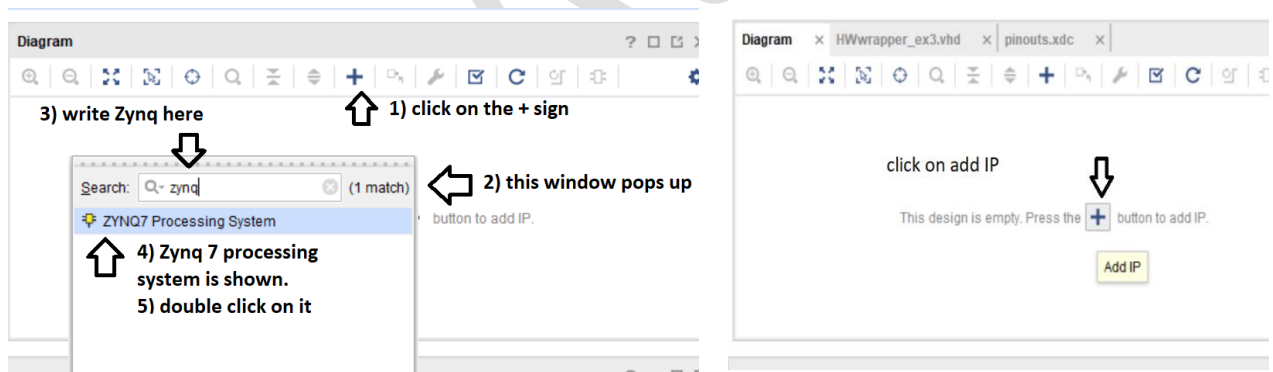
Figure 21: Including the Processing System
